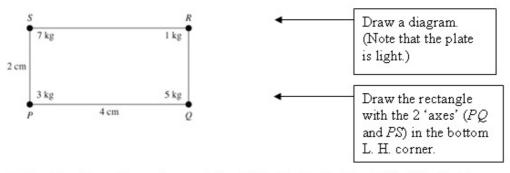
Taking P as the origin, and axes, PQ and PS, P is (0, 0); Q is (4, 0); R is (4, 2); S is (0, 2).
