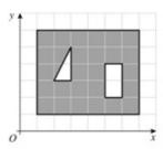
The diagram shows a uniform plane figure drawn on a grid of unit squares. Find the coordinates of the centre of mass.
