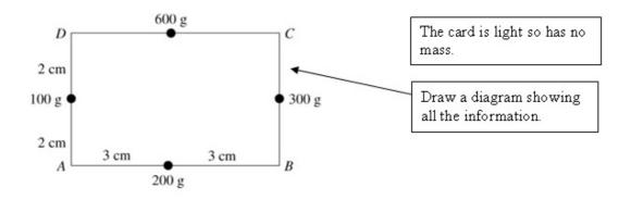
Taking axes through A, the coordinates of the masses are (3, 0), (6, 2), (3, 4) and (0, 2).
